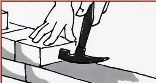
Tap brick firmly with hammer against side as shown.
