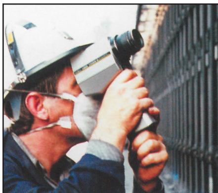
The oven temperature is carefully monitored to ensure optimum ceramic welding conditions as well as protecting the oven from further damage.
