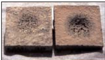
Figure 2: C-704 abrasion plates show that R-MAX® C (left) has less than half the abrasion loss of typical low cement castable (right).
