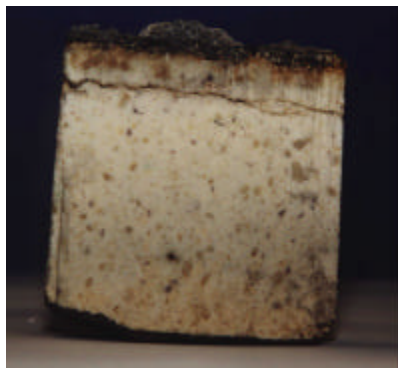
Figure four: Cut section of the brick shows cracking below the hot face portion where the liquid phase has penetrated.
