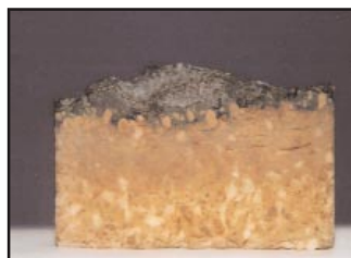
Liquid phase attack at the hot face of a conventional magnesite-spinel brick changes the refractory structure and leads to erosion, cracking and spalling.
