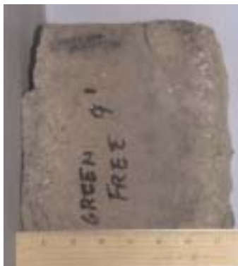
Figure 1. GREENFREE™ KF was approximately 180-mm (7") thick after the first campaign in the lower transition of a 12' diameter cement kiln.
