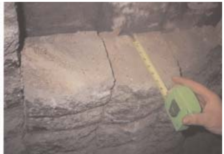
Figure 2. RESCOMAG® 92 FMS exhibited superior erosion resistance and good remnant thickness after its campaign in a 4.4-m diameter kiln.
