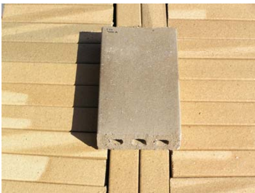
Comparisons of Surface Color from Roller Hearth vs. Periodic (Bee Hive) Firing
