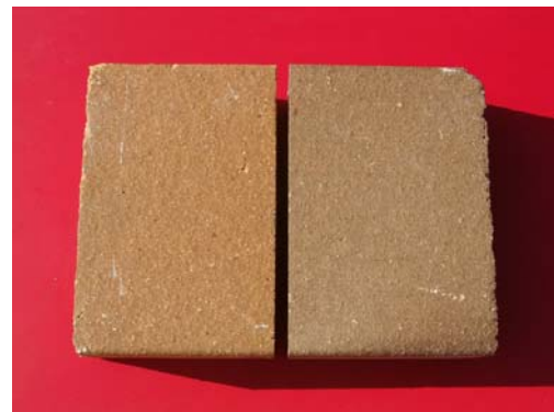
Comparisons of Surface Color from Roller Hearth vs. Periodic (Bee Hive) Firing
