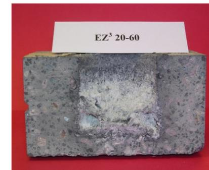
**Figure 6.** EZ CUBED® 20-60 contains about 60% silicon carbide. In the alkali cup test, no cracking was observed. The test cup indicates some reaction with the alkali.
