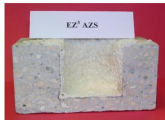
Figure 8. EZ CUBED® AZS is widely used in linings where buildup management is desired. This product contains about 5% silicon carbide receives an excellent rating in the alkali cup test.
