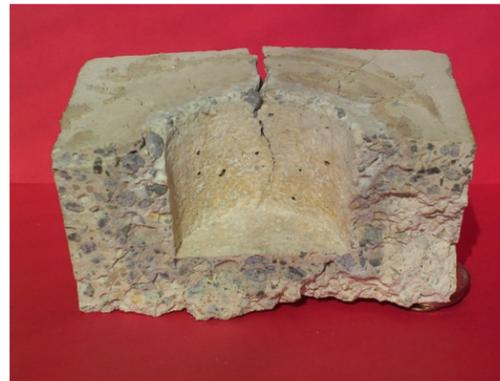
**Figure 2.** Alkali cup test of 80% alumina castable shows cracking from expansive phases formed and discoloration due to penetration.
