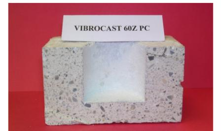
**Figure 4.** VIBROCAST 60Z PC alkali cup test exhibits exceptional resistance, no penetration and a very clean cup.
