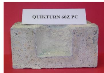
Figure 9. Alkali cup test of QUIKTURN™ 60Z PC shows no cracking, minor penetration and overall excellent alkali resistance.
