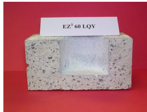
**Figure 3.** EZ CUBED® 60 LQY is a 55% alumina shotcrete castable with outstanding alkali resistance.
