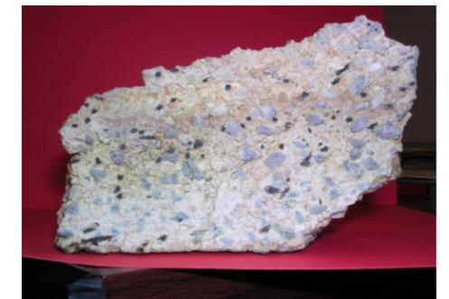
Figure 1. Alkali attack in a high alumina castable caused cracking and friability in the refractory. Alkali reactions have discolored the grains and caused expansive growth.
