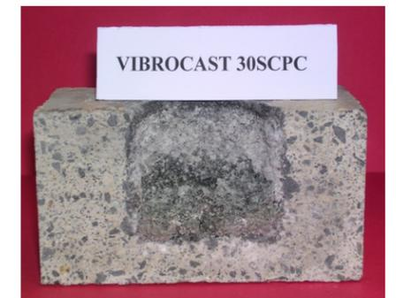
**Figure 7.** VIBROCAST® 30SCPC is an example of a medium SiC content product that receives a very good rating in the alkali cup test. No cracking detected and moderate penetration.
