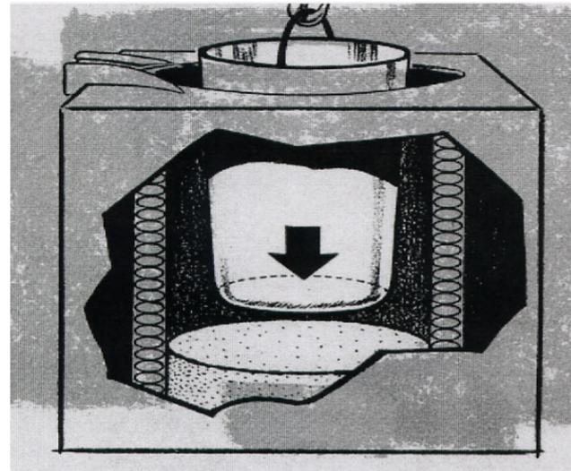
**To provide equal wall thickness, the burnout form should be centered**
