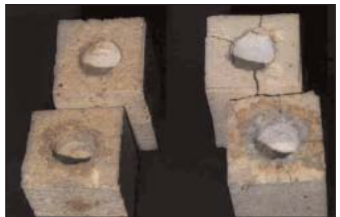
Figure 3. SENECA™ 60P (left) exhibits superior resistance to alkali cracking in laboratory cup test.
